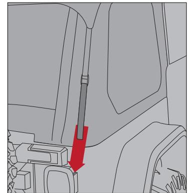
13. Pull roof top down. Handle metal hooks on end of straps with care to avoid damage or injury. Attach flat hooks under Belt Rail at reinforced patches on each side of tailgate; pull straps down snugly. While holding straps in line and secured to the hook and loop, close the cam buckle into the locked position.
